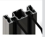
Double glazed mullion will accept two monolithic sheets of glass up to 12.50mm thick. This creates approximately 44mm gap between for improved acoustic performance.
